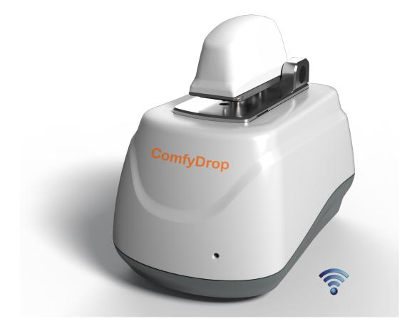
ComfyDrop<sup>™</sup> gives highly accurate full spectrum measurements with micro-samples (spectrum range: 185 - 910nm). ComfyDrop<sup>™</sup> is widely used in molecular biological experiments and in absorbance detection for the general substance analysis.
